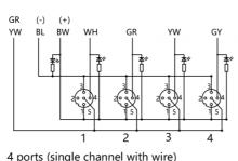
4 ports (single channel with wire) NPN Circuit schematic
