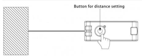
(2) Press the teaching button for more than 3 seconds until the traffic light flashes alternately. Release the button to complete teaching.
