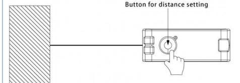
(2) Press the teaching button for more than 3 seconds until the traffic light flashes alternately. Release the button to complete teaching.
